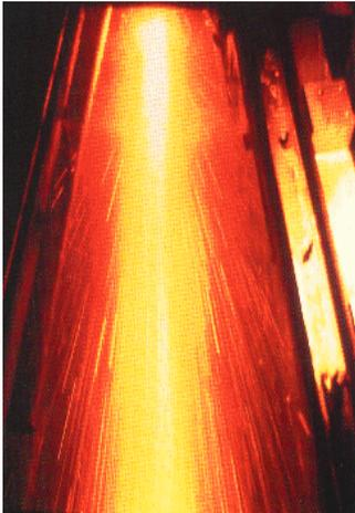
Atomization of molten metal in the CPM process
