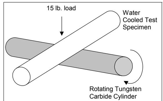
Fig. 1 Picture of cross cylinder wear test
